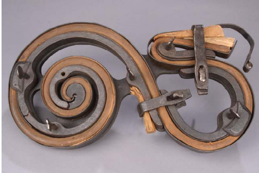
Figure 4. Example of stages of processing: a bentwood furniture molding press for a sofa, around 1900
